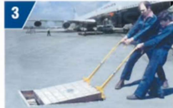
3 Slide back the cover on EZI-LIFT rollers
