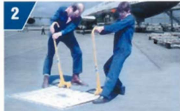
2 Gently pull back the EZI-LIFT's to raise one edge of the cover
