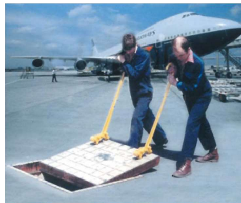
6 Turn the EZI-LIFT through 180° to slide the cover back into place to re seat
