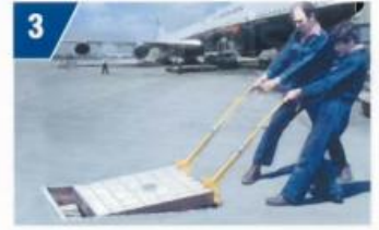
3 Slide back the cover on EZI-LIFT rollers
