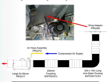
The Large Air Mover Kit can be configured to accommodate almost any aircraft configuration.
